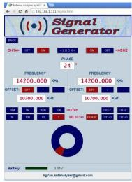
two independent channels with a frequency resolution of 1 Hz. Moreover, the relative phase shift between signals of the two channels can be controlled by 1 degree increments from 0 to 360 degrees. Perhaps the most interesting part of the instrument is the control and
