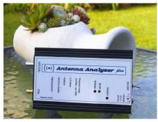
panel size is 115 x 75 mm fitting into a small box of size eg. 125 x 80 x 25 mm. Its main function is put into effect by the two RF impedance meters - called together the antenna analyzer - which can measure phase true complex impedance between the main
